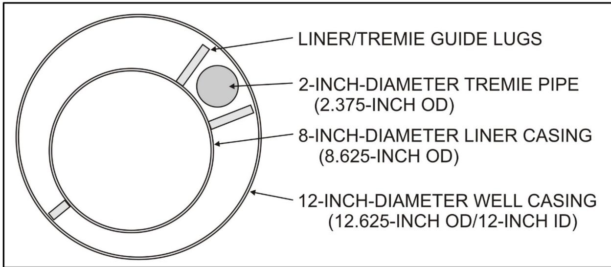
**Figure 3 – Tremie and Liner Guide Lug Placement**
