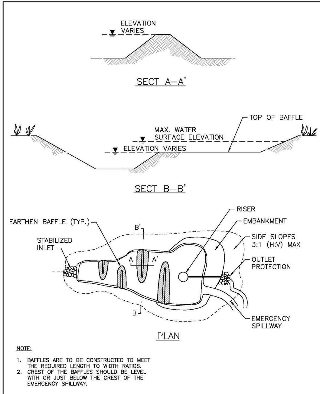
**FIGURE 4: TYPICAL TEMPORARY SEDIMENT BASIN WITH BAFFLES**
