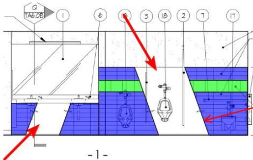
these are called "cut lines". it is a standard architectural drawing method to not draw an entire pattern for ease of clarity and for less drawing. the tile patterns colored green and blue are continuous.
